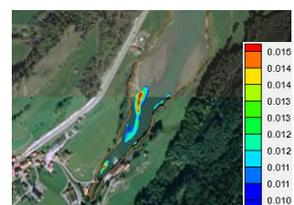
Fig. 4: Lake Lessoc. Deposition difference between current and future state for turbinage of 40 m<sup>3</sup>/s during 48 hours.
