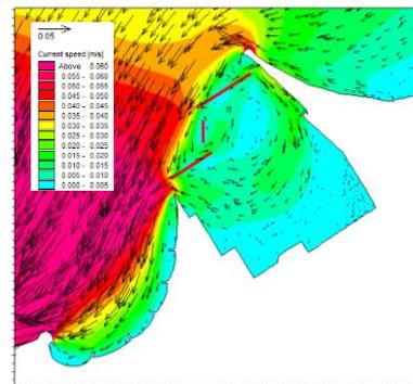
Fig. 2: Velocity field for the curved triangular beach alternative with a discharge of 250 m<sup>3</sup>/s at Seujet dam.
